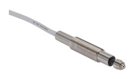
Metrol limit switch, precision touch, 8mm diameter, threaded, 0.75mm pitch, 52.8mm length, 2mm round head, stainless steel, 5.5mm plunger, 1N contact force, N.O. contact(s), 9.8ft/3m cable length, pigtail.
