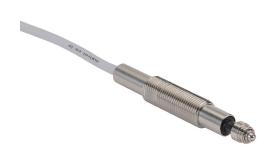
Metrol limit switch, precision touch, 8mm diameter, threaded, 0.75mm pitch, 52.8mm length, 2mm round head, stainless steel, 5.5mm plunger, 1N contact force, (1) N.O. contact(s), 9.8ft/3m cable length, pigtail.
