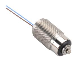
Metrol limit switch, precision touch, 10mm diameter, threaded, 0.5mm pitch, 20.5mm length, 2.5mm radius head, stainless steel, 2mm plunger with boot, 1N contact force, (1) N.O. contact(s), 1.6ft/0.5m cable length, core wire.
