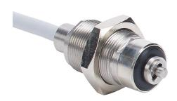
Metrol limit switch, precision touch, 10mm diameter, threaded, 0.5mm pitch, 24.7mm length, 2.5mm radius head, stainless steel, 2mm plunger with boot, 1N contact force, (1) N.O. contact(s), 6.5ft/2m cable length, pigtail.
