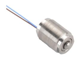
Metrol limit switch, precision touch, 10mm diameter, threaded, 0.5mm pitch, 15mm length, 2.5mm radius head, stainless steel, 3.5mm plunger, 1N contact force, N.O. contact(s), 1.6ft/0.5m cable length, core wire.
