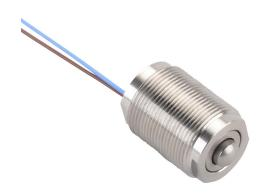
Metrol limit switch, precision touch, 10mm diameter, threaded, 0.5mm pitch, 15mm length, 2.5mm radius head, stainless steel, 3.5mm plunger, 1N contact force, (1) N.O. contact(s), 1.6ft/0.5m cable length, core wire.
