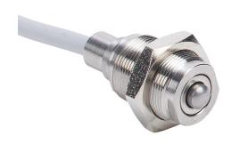
Metrol limit switch, precision touch, 10mm diameter, threaded, 0.5mm pitch, 21.5mm length, 2.5mm radius head, stainless steel, 3.5mm plunger, 1N contact force, (1) N.O. contact(s), 6.5ft/2m cable length, pigtail.
