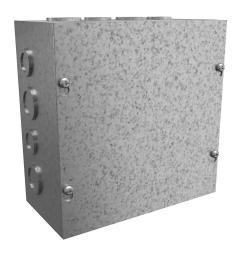
Hammond enclosure, NEMA 1, 8 x 8 x 4in (HxWxD), wall mount, with knockouts, galvanized steel, screw cover.
