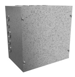
Hammond enclosure, NEMA 1, 12 x 12 x 8in (HxWxD), wall mount, with knockouts, galvanized steel, screw cover.
