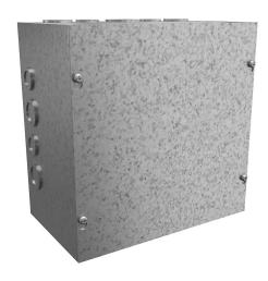
Hammond enclosure, NEMA 1,  $10 \times 10 \times 6$ in (HxWxD), wall mount, with knockouts, galvanized steel, screw cover.
