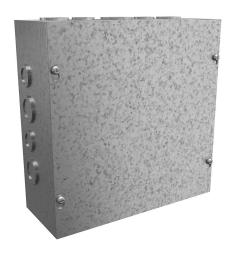
Hammond enclosure, NEMA 1,  $10 \times 10 \times 4$ in (HxWxD), wall mount, with knockouts, galvanized steel, screw cover.
