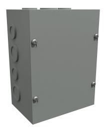
Hammond enclosure, NEMA 1, 8 x 6 x 4in (HxWxD), wall mount, with knockouts, carbon steel, ANSI 61 gray, powder coat finish, screw cover.
