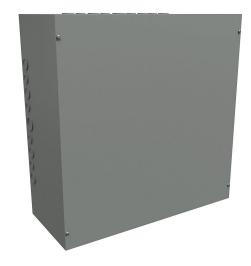
Hammond enclosure, NEMA 1,  $24 \times 24 \times 10$  in (HxWxD), wall mount, with knockouts, carbon steel, ANSI 61 gray, powder coat finish, screw cover.
