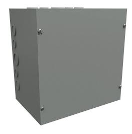
Hammond enclosure, NEMA 1,  $12 \times 12 \times 8$ in (HxWxD), wall mount, with knockouts, carbon steel, ANSI 61 gray, powder coat finish, screw cover.
