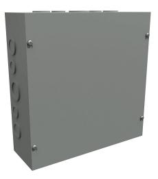
Hammond enclosure, NEMA 1, 12 x 12 x 4in (HxWxD), wall mount, with knockouts, carbon steel, ANSI 61 gray, powder coat finish, screw cover.
