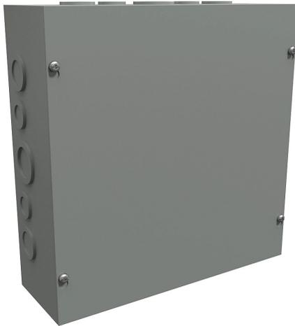
Hammond enclosure, NEMA 1, 12 x 12 x 4in (HxWxD), wall mount, with knockouts, carbon steel, ANSI 61 gray, powder coat finish, screw cover.
