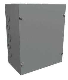
Hammond enclosure, NEMA 1,  $12 \times 10 \times 6$ in (HxWxD), wall mount, with knockouts, carbon steel, ANSI 61 gray, powder coat finish, screw cover.
