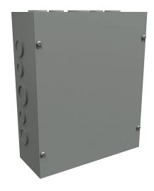
Hammond enclosure, NEMA 1,  $12 \times 10 \times 4$ in (HxWxD), wall mount, with knockouts, carbon steel, ANSI 61 gray, powder coat finish, screw cover.
