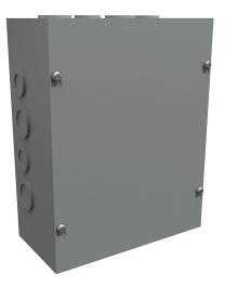
Hammond enclosure, NEMA 1, 10 x 8 x 4in (HxWxD), wall mount, with knockouts, carbon steel, ANSI 61 gray, powder coat finish, screw cover.
