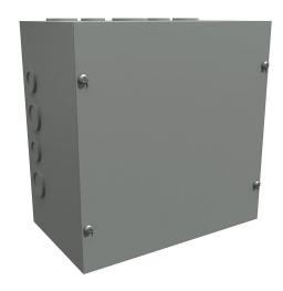
Hammond enclosure, NEMA 1,  $10 \times 10 \times 6$ in (HxWxD), wall mount, with knockouts, carbon steel, ANSI 61 gray, powder coat finish, screw cover.
