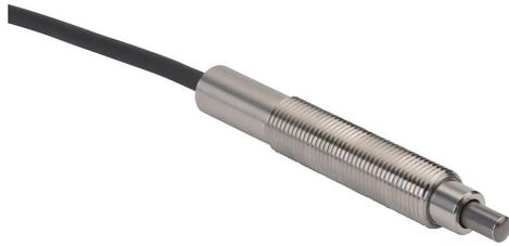
Metrol limit switch, precision touch, 8mm diameter, threaded, 0.75mm pitch, 54.5mm length, 3mm radius head, stainless steel, 3.5mm plunger, 1N contact force, (1) N.C. contact(s), 9.8ft/3m cable length, pigtail.
