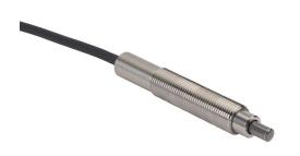
Metrol limit switch, precision touch, 8mm diameter, threaded, 0.75mm pitch, 54.5mm length, 3mm radius head, stainless steel, 3.5mm plunger, 1N contact force, (1) N.C. contact(s), 9.8ft/3m cable length, pigtail.
