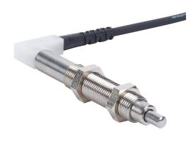
Metrol limit switch, precision touch, 8mm diameter, threaded, 0.75mm pitch, 66.2mm length, 3mm radius head, stainless steel, 3.5mm plunger, 1N contact force, N.C. contact(s), 9.8ft/3m cable length, 90 degree exit, pigtail.
