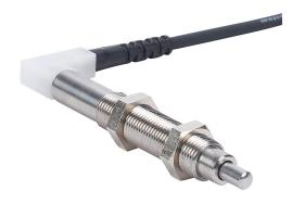
Metrol limit switch, precision touch, 8mm diameter, threaded, 0.75mm pitch, 66.2mm length, 3mm radius head, stainless steel, 3.5mm plunger, 1N contact force, (1) N.C. contact(s), 9.8ft/3m cable length, 90 degree exit, pigtail.
