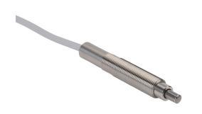
Metrol limit switch, precision touch, 8mm diameter, threaded, 0.75mm pitch, 54.5mm length, 3mm radius head, stainless steel, 3.5mm plunger, 1N contact force, (1) N.O. contact(s), 9.8ft/3m cable length, pigtail.
