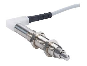
Metrol limit switch, precision touch, 8mm diameter, threaded, 0.75mm pitch, 66.2mm length, 3mm radius head, stainless steel, 3.5mm plunger, 1N contact force, (1) N.O. contact(s), 9.8ft/3m cable length, 90 degree exit, pigtail.
