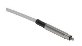
Metrol limit switch, precision touch, 5mm diameter, smooth, 42mm length, 1.5mm radius head, stainless steel, 2mm plunger, 1N contact force, (1) N.O. contact(s), 9.8ft/3m cable length, pigtail.
