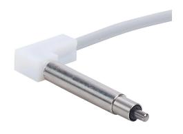
Metrol limit switch, precision touch, 5mm diameter, smooth, 40mm length, 1.5mm radius head, stainless steel, 2mm plunger, 1N contact force, (1) N.O. contact(s), 9.8ft/3m cable length, 90 degree exit, pigtail.
