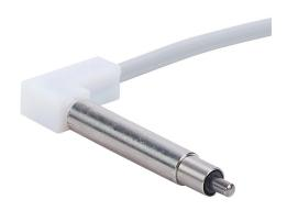
Metrol limit switch, precision touch, 5mm diameter, smooth, 40mm length, 1.5mm radius head, stainless steel, 2mm plunger, 1N contact force, N.O. contact(s), 9.8ft/3m cable length, 90 degree exit, pigtail.
