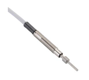
Metrol limit switch, precision touch, 5mm diameter, threaded, 0.5mm pitch, 55.5mm length, 1.5mm flat head, stainless steel, needle plunger, 1N contact force, (1) N.O. contact(s), 9.8ft/3m cable length, pigtail.
