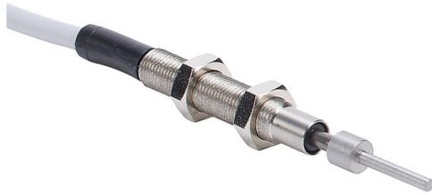
Metrol limit switch, low contact force, precision touch, 5mm diameter, threaded, 0.5mm pitch, 55.5mm length, 1.5mm flat head, stainless steel, needle plunger, 0.5N contact force, (1) N.O. contact(s), 9.8ft/3m cable length, pigtail.
