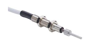
Metrol limit switch, low contact force, precision touch, 5mm diameter, threaded, 0.5mm pitch, 55.5mm length, 1.5mm flat head, stainless steel, needle plunger, 0.5N contact force, (1) N.O. contact(s), 9.8ft/3m cable length, pigtail.
