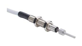
Metrol limit switch, low contact force, precision touch, 5mm diameter, threaded, 0.5mm pitch, 55.5mm length, 1.5mm flat head, stainless steel, needle plunger, 0.5N contact force, N.O. contact(s), 9.8ft/3m cable length, pigtail.
