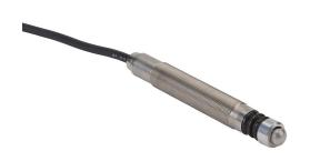
Metrol limit switch, sliding/angled, precision touch, 8mm diameter, threaded, 0.5mm pitch, 62.5mm length, 3mm radius head, stainless steel, 4.7mm plunger, 1N contact force, (1) N.C. contact(s), 6.5ft/2m cable length, pigtail.
