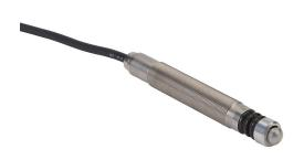
Metrol limit switch, sliding/angled, precision touch, 8mm diameter, threaded, 0.5mm pitch, 62.5mm length, 3mm radius head, stainless steel, 4.7mm plunger, 1N contact force, N.C. contact(s), 6.5ft/2m cable length, pigtail.
