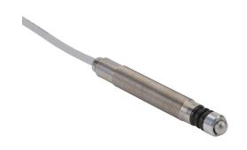
Metrol limit switch, sliding/angled, precision touch, 8mm diameter, threaded, 0.5mm pitch, 62.5mm length, 3mm radius head, stainless steel, 4.7mm plunger, 1N contact force, (1) N.O. contact(s), 6.5ft/2m cable length, pigtail.
