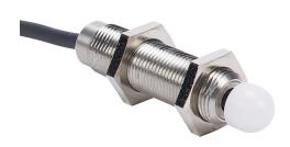
Metrol limit switch, sliding/angled, precision touch, 12mm diameter, threaded, 1mm pitch, 59.5mm length, 5mm radius head, plastic, 10mm plunger, 1.5N contact force, (1) N.C. contact(s), 6.5ft/2m cable length, pigtail.
