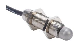
Metrol limit switch, sliding/angled, precision touch, 12mm diameter, threaded, 1mm pitch, 59.5mm length, 5mm radius head, stainless steel, 10mm plunger, 1.5N contact force, (1) N.C. contact(s), 6.5ft/2m cable length, pigtail.
