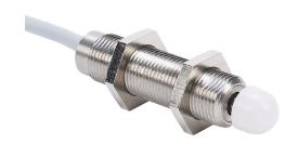
Metrol limit switch, sliding/angled, precision touch, 12mm diameter, threaded, 1mm pitch, 59.5mm length, 5mm radius head, plastic, 10mm plunger, 1.5N contact force, (1) N.O. contact(s), 6.5ft/2m cable length, pigtail.
