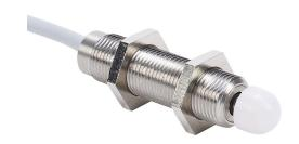
Metrol limit switch, sliding/angled, precision touch, 12mm diameter, threaded, 1mm pitch, 59.5mm length, 5mm radius head, plastic, 10mm plunger, 1N contact force, N.O. contact(s), 6.5ft/2m cable length, pigtail.
