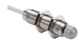
Metrol limit switch, sliding/angled, precision touch, 12mm diameter, threaded, 1mm pitch, 59.5mm length, 5mm radius head, stainless steel, 10mm plunger, 1.5N contact force, (1) N.O. contact(s), 6.5ft/2m cable length, pigtail.
