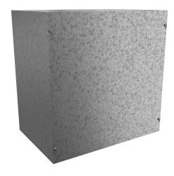
Hammond enclosure, NEMA 1, 18 x 18 x 12in (HxWxD), wall mount, galvanized steel, screw cover.
