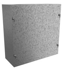
Hammond enclosure, NEMA 1, 10 x 10 x 4in (HxWxD), wall mount, galvanized steel, screw cover.
