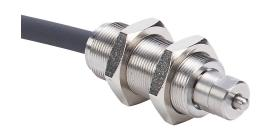
Metrol limit switch, precision touch, 10mm diameter, threaded, 0.5mm pitch, 30mm length, 1.5mm radius head, stainless steel, 2mm plunger, 0.1N contact force, NPN, N.O., 9.8ft/3m cable length, pigtail.
