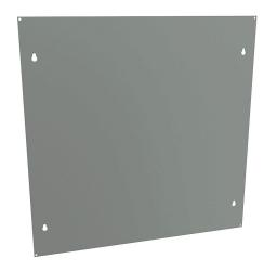
Hammond flush cover, carbon steel, 16 gauge, ANSI 61 gray, powder coat finish. For use with 18 x 18in (HxW) CS and CSKO screw cover enclosures.
