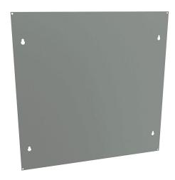
Hammond flush cover, carbon steel, 16 gauge, ANSI 61 gray, powder coat finish. For use with 16 x 16in (HxW) CS and CSKO screw cover enclosures.
