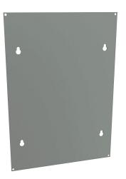
Hammond flush cover, carbon steel, 16 gauge, ANSI 61 gray, powder coat finish. For use with 12 x 8in (HxW) CS and CSKO screw cover enclosures.
