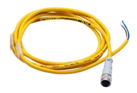
Cable, M12 axial female to pigtail, 4-pole, PVC jacket, yellow, 6.5ft/2m cable length, IP67.
