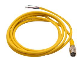
AC micro cable, 1/2in-20 UNF thread axial female to pigtail, 5-pole, PVC jacket, yellow, 6.5ft/2m cable length, IP67.
