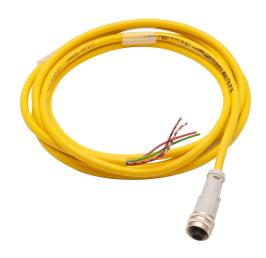
AC micro cable, 1/2in-20 UNF thread axial female to pigtail, 4-pole, PVC jacket, yellow, 6.5ft/2m cable length, IP67.
