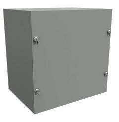
Hammond enclosure, NEMA 1, 8 x 8 x 6in (HxWxD), wall mount, carbon steel, ANSI 61 gray, powder coat finish, screw cover.
