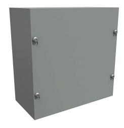
Hammond enclosure, NEMA 1, 8 x 8 x 4in (HxWxD), wall mount, carbon steel, ANSI 61 gray, powder coat finish, screw cover.
