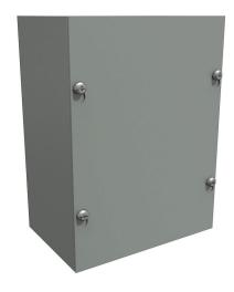
Hammond enclosure, NEMA 1, 8 x 6 x 4in (HxWxD), wall mount, carbon steel, ANSI 61 gray, powder coat finish, screw cover.
