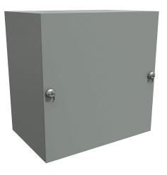
Hammond enclosure, NEMA 1, 6 x 6 x 4in (HxWxD), wall mount, carbon steel, ANSI 61 gray, powder coat finish, screw cover.
