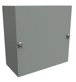
Hammond enclosure, NEMA 1, 6 x 6 x 3in (HxWxD), wall mount, carbon steel, ANSI 61 gray, powder coat finish, screw cover.
