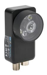
di-soric CS60 series 2D vision camera, 50-515mm operating distance, localization, detection, counting and measurement, 1440 x 1080 resolution, white and red light emission, TCP/IP, FTP Client, SFTP Client, Profinet Client and EtherNet/IP Client, IP67.
