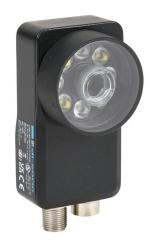
di-soric CS60 series 2D vision camera, 50-515mm operating distance, localization, detection, counting, read code, and measurement, 1440 x 1080 resolution, white and red light emission, TCP/IP, FTP Client, SFTP Client, Profinet Client and EtherNet/IP Client, IP67.
