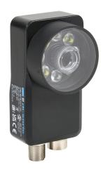
di-soric CS60 series 2D vision camera, 50-515mm operating distance, localization, detection and counting, 1440 x 1080 resolution, white and red light emission, TCP/IP, FTP Client, SFTP Client, Profinet Client and EtherNet/IP Client, IP67.
