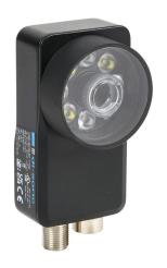
di-soric CS60 series 2D vision camera, 50-515mm operating distance, localization, detection and counting, 736 x 480 resolution, white and red light emission, TCP/IP, FTP Client, SFTP Client, Profinet Client and EtherNet/IP Client, IP67.
