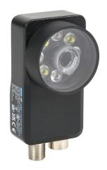
di-soric CS60 series 2D vision camera, 50-515mm operating distance, localization, detection, counting and read code, 736 x 480 resolution, white and red light emission, TCP/IP, FTP Client, SFTP Client, Profinet Client and EtherNet/IP Client, IP67.
